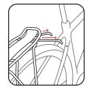
Reach the arms forward to the seat stay eyelets. The arms may reach better with the 90° angle pointing toward the inside or outside of the frame, either way will work.
