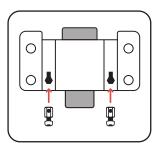
Insert the nuts into the adapter with the holes aligned vertically.
