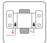
Pull down the cable ends to equal length (min. 2cm) and bend them towards the center.
