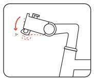
Push the adapter downwards until it is stopped by the cable. The adapter should be tilted upwards slightly. If necessary, loosen one bolt to adjust. Tighten the four black screws holding the clamps (1.5 Nm).
